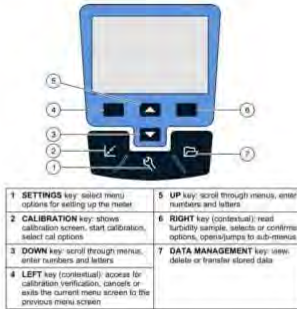
Figure 15: Hach turbidity meter button options
