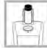
2. Gently invert the standard. Insert the 10.0 NTU (or other defined value) Verification Standard and close the lid.
