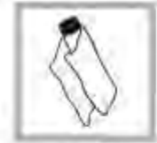
3. Use the provided oiling cloth to spread the oil uniformly. Wipe off the excess so that only a thin coat of oil is left. Make sure that the sample cell is almost dry with little or no visible oil. Note: Store the oiling cloth in a plastic storage bag to keep the cloth clean.
