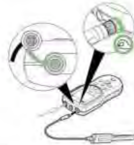
Figure 8: Connecting the probes to the meter.
