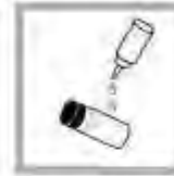
2. Apply a small bead of silicone oil from the top to the bottom of the cell.
