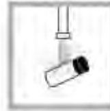
1. Clean the inside and outside of the cell and caps by washing with a laboratory glass cleaning detergent. Follow with multiple rinses with distilled or demineralized water.
