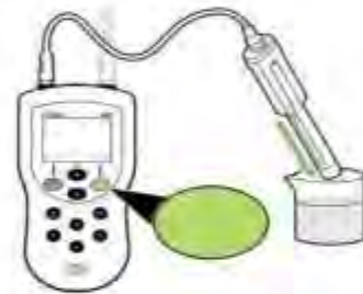
Figure 10: Press the green button to stabilize readings
