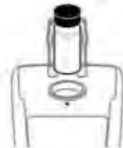
Figure 14: Insert vial into center by aligning the arrows
