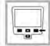
3. Push Read . The display shows Stabilizing and then shows the result and tolerance range.
