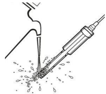
Figure 15: Rinse the probe with DI water
