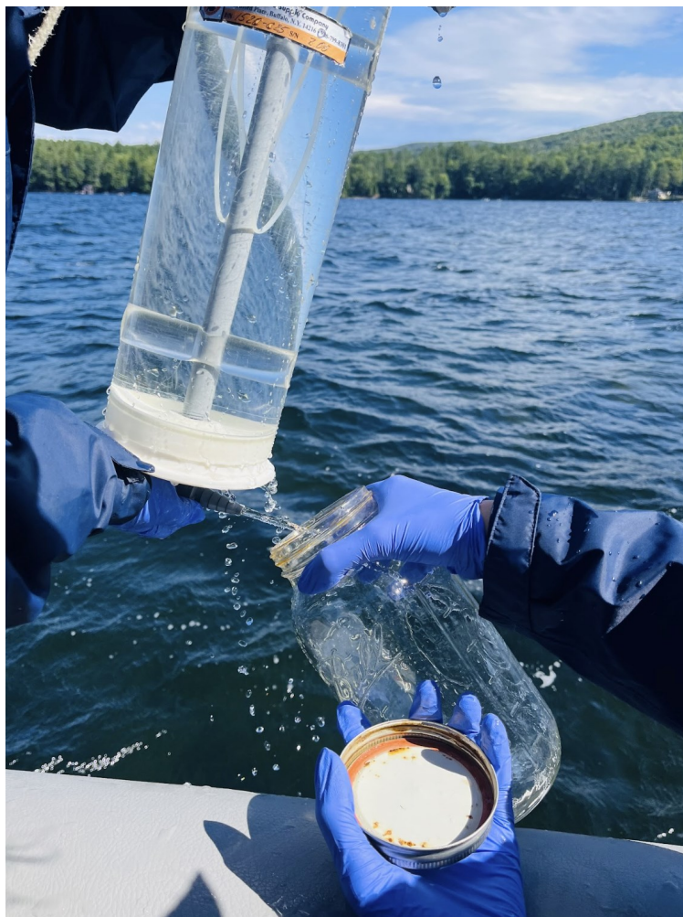
To collect eDNA samples in deep water, a decontaminated Van Dorn is used (L). The sample is then transferred into a decontaminated container (R). These samples are brought back to the GMCG research center for DNA extraction and analysis.
