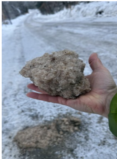
A large chunk of road salt found after winter maintenance highlights how oversalting can occur in a concentrated location when salt is not properly dispersed.
